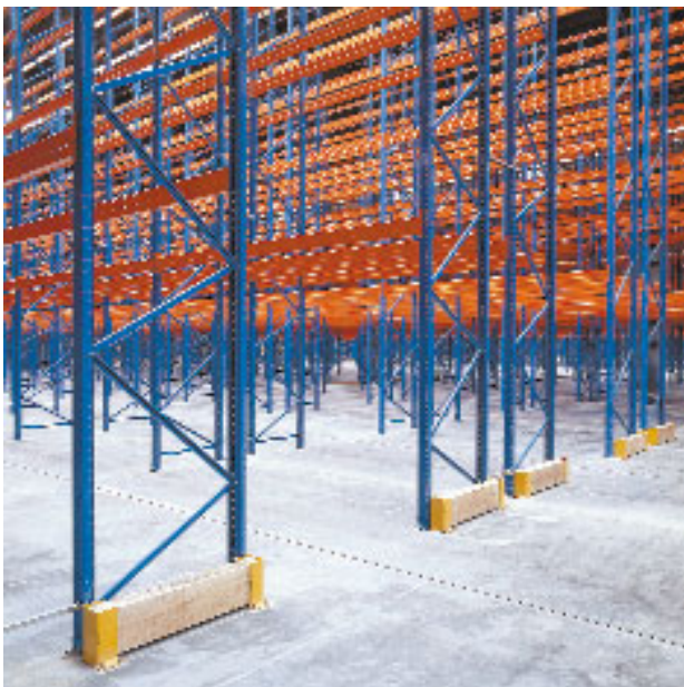
A typical arrangement from the Static Storage Systems Division (Stow): Stow elements manufactured in automated, high-volume production plants form the core of a customized high-bay warehouse solution.
