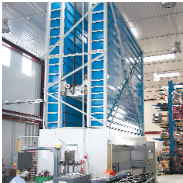
A typical solution from the Special-Purpose Handling Systems Division (STE): an STE multi-tower for heavy loads is used for the centralized storage of long, flat items up to 6.8 m.
